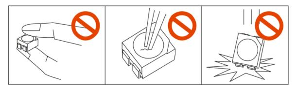
2. The epoxy resin of encapsulant is fragile, so please avoid scratch or friction over the epoxy resin surface. While handling the product with tweezers, do not hold by the epoxy resin, be careful.
