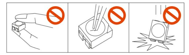
2. The epoxy resin of encapsulant is fragile, so please avoid scratch or friction over the epoxy resin surface. While handling the product with tweezers, do not hold by the epoxy resin, be careful.
